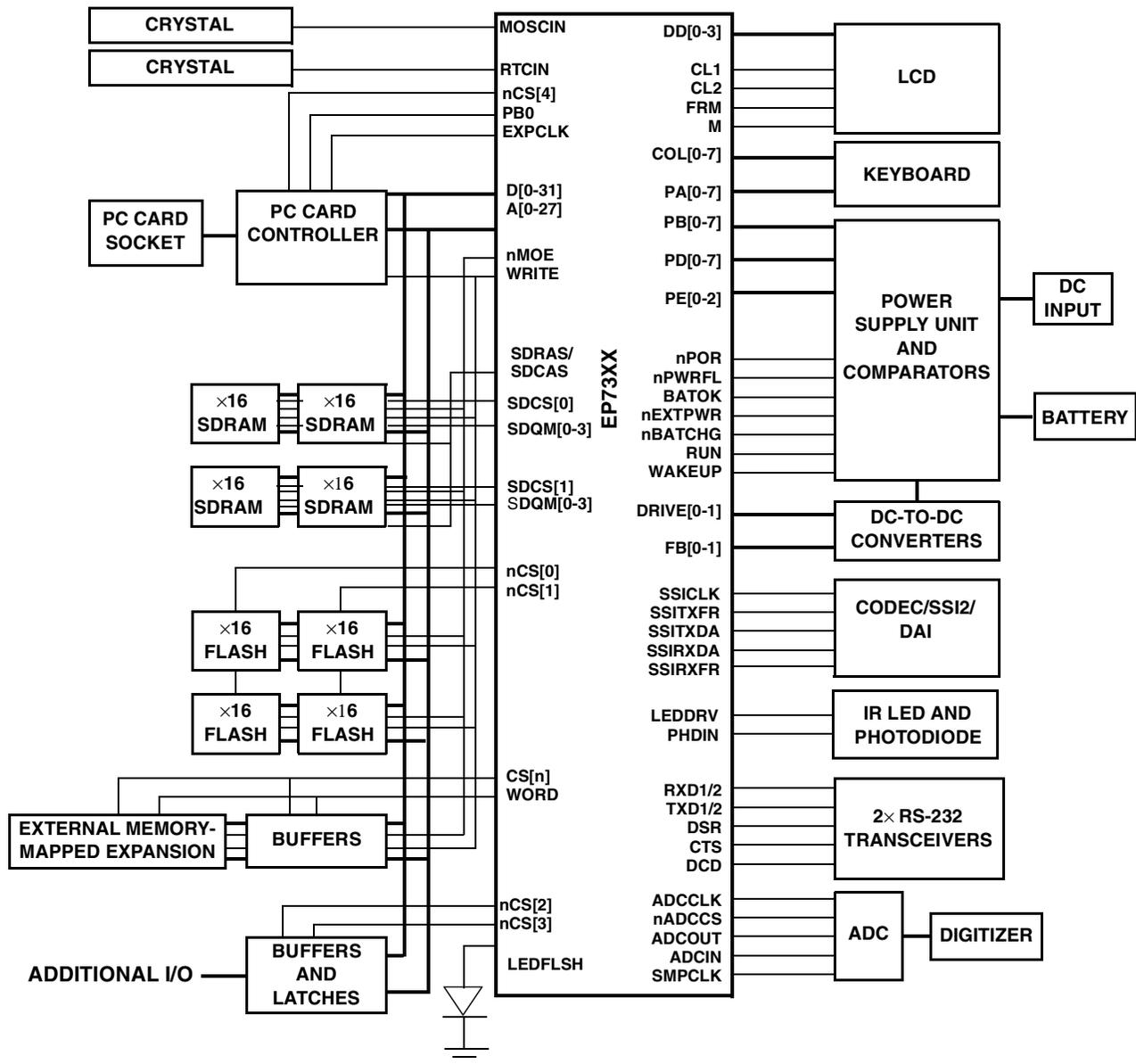
Figure 1-2. Typical EP73xx System Block Diagram
