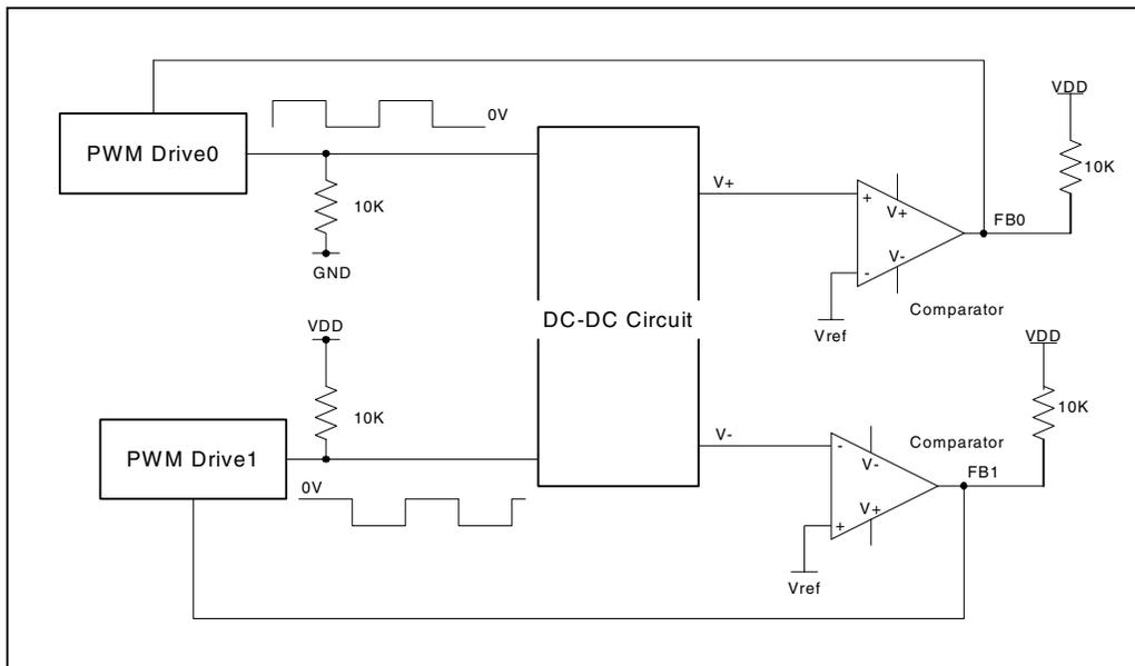
Figure 12-1. Block Diagram of a Power Supply Using Two PWM Drives
