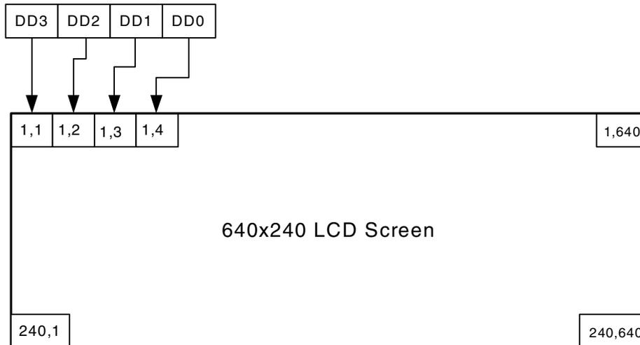
Figure 9-2. LCD Data to Pixel Mapping
