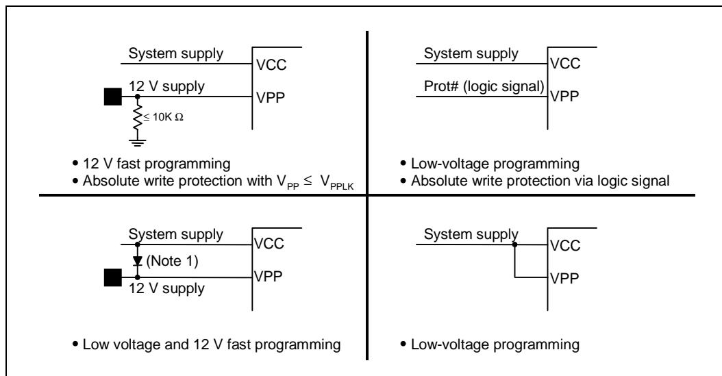
**NOTE:** If the  $V_{CC}$  supply can sink adequate current, you can use an appropriately valued resistor.
