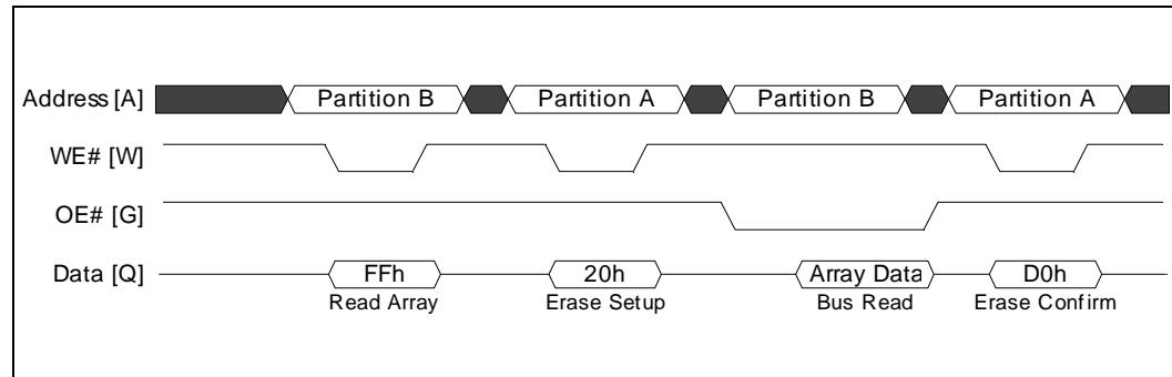
By contrast, a write bus cycle may not interrupt a 2-cycle write sequence. Doing so causes a command sequence error to appear in the status register. [Figure 4](#) illustrates a command sequence error.
