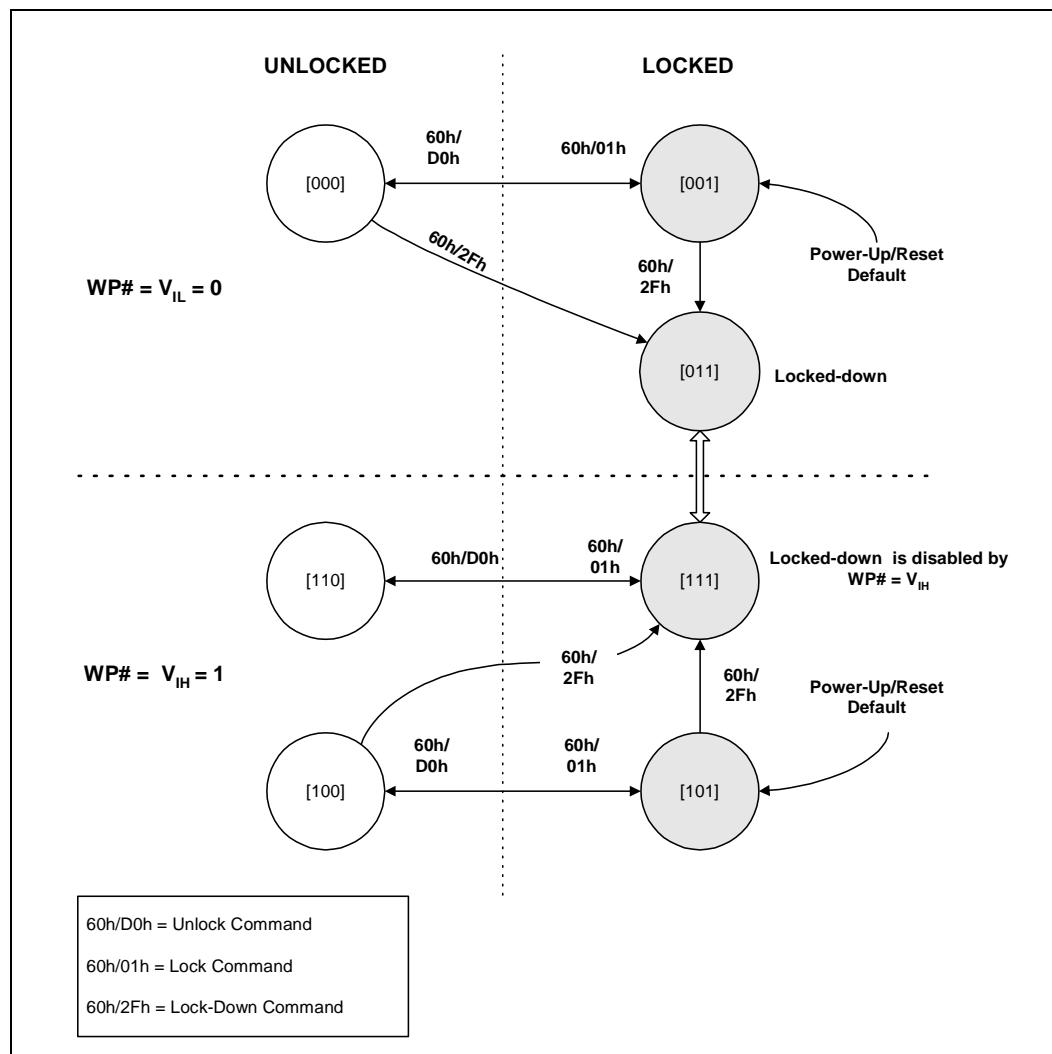
**NOTE:** The notation [X,Y,Z] denotes the locking state of a block. The current locking state of a block is defined by the state of WP# and the two bits of the block-lock status D[1:0].
