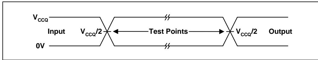
NOTE: Input timing begins, and output timing ends, at  $V_{CCQ}/2$ . Input rise and fall times (10% to 90%) < 5 ns.
